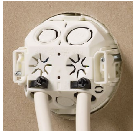
Ø 16 mm pipe entries can be used for cable. Strips are used as strain reliefs.
