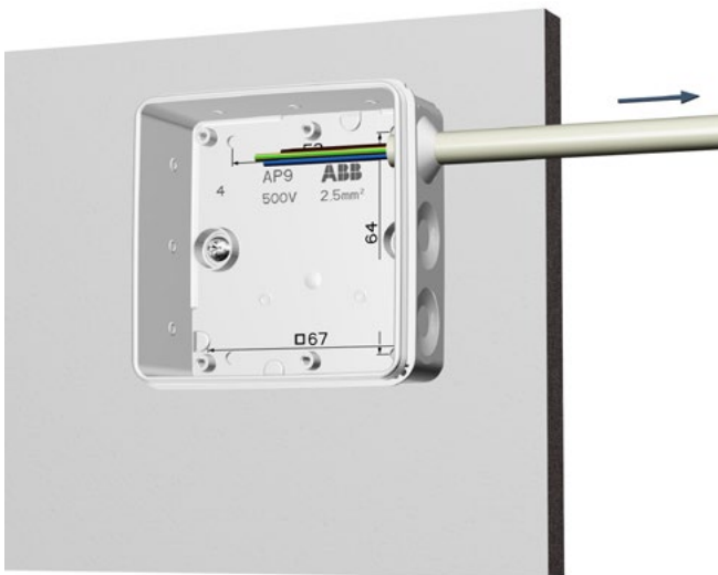
Pull cable back to seal entry. Box enclosure class IP55/IP65. There are draining holes at the bottom of the box which can be opened in case of extreme weather conditions.
